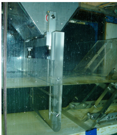
Figure 3: Photograph of the OWSC model in the 2D wave flume
